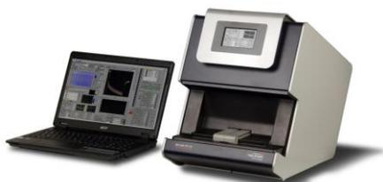
Microscale Thermophoresis is based on a physical principle, used for the first time for biomolecular interaction studies. It measures changes of the mobility of molecules in microscopic temperature gradients. The technology is exceptional sensitive since it detects changes in size, charge and hydration shell of molecules. NanoTemper provides two Monolith series instruments based on MST:
